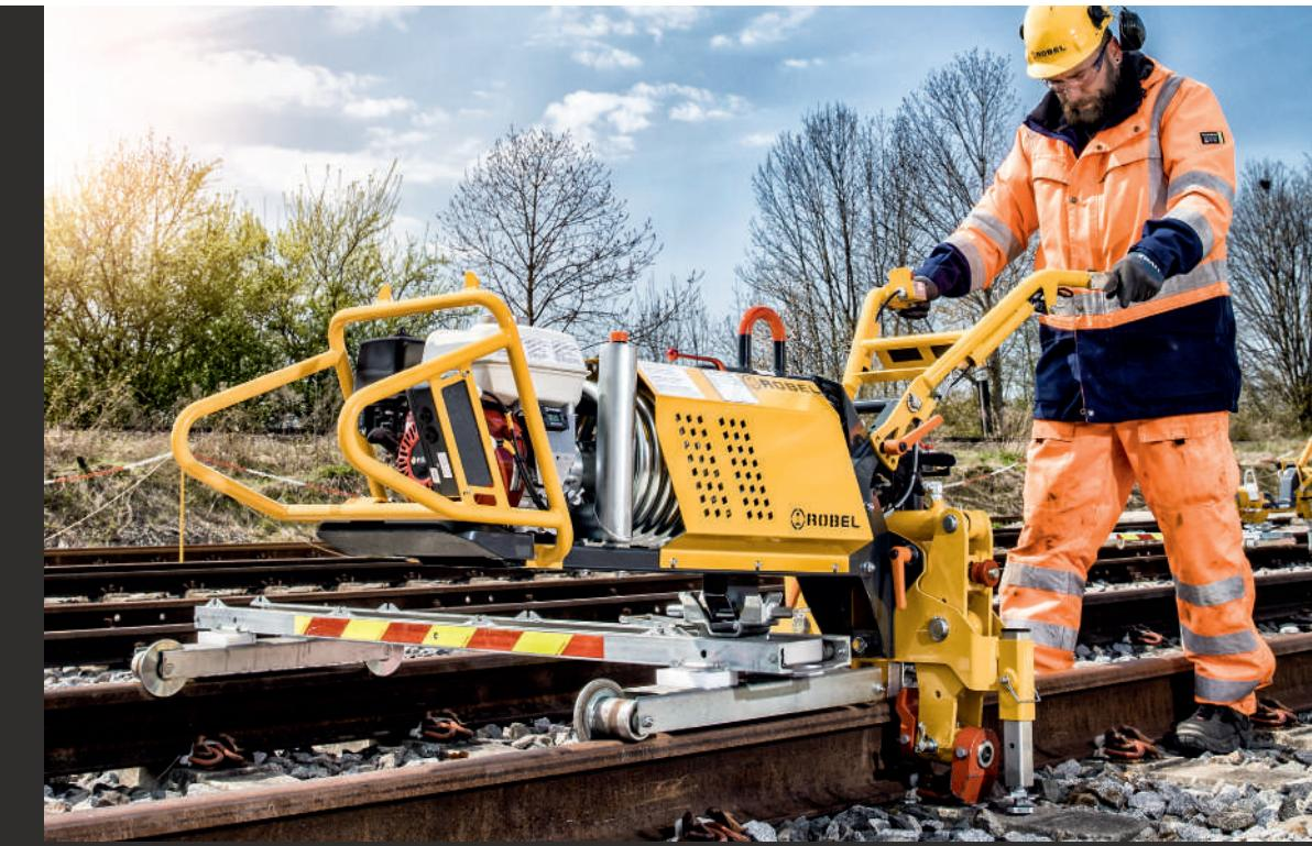
For inserting and extracting Fastclip clips, including tie lifting piston.
