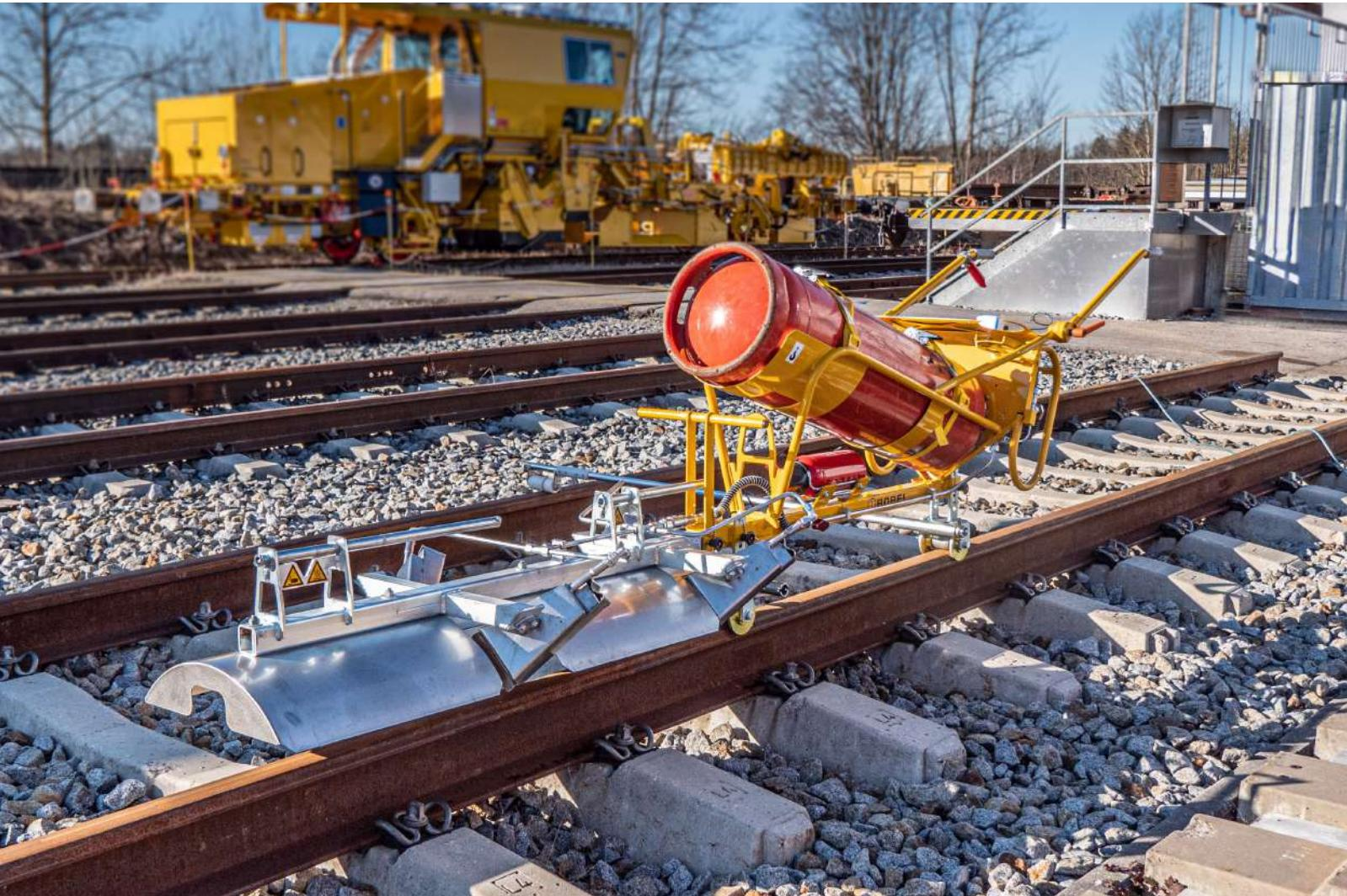
Designed to create the nominal rail temperature before welding.
