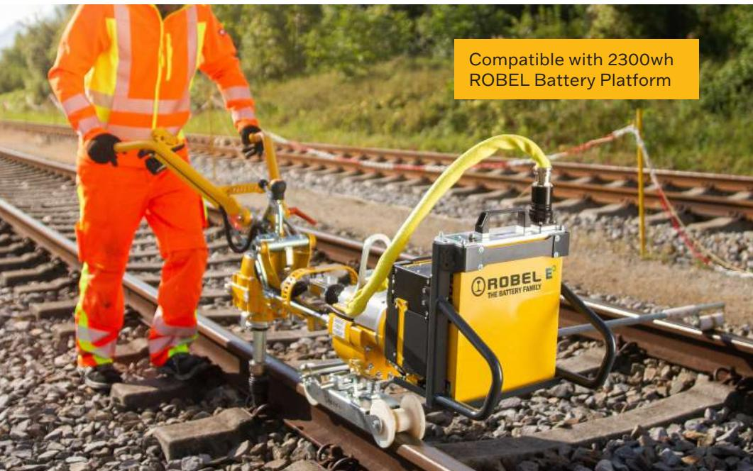
**Production-grade machine for tightening and loosening of tie, switch, and joint bar bolts.**
