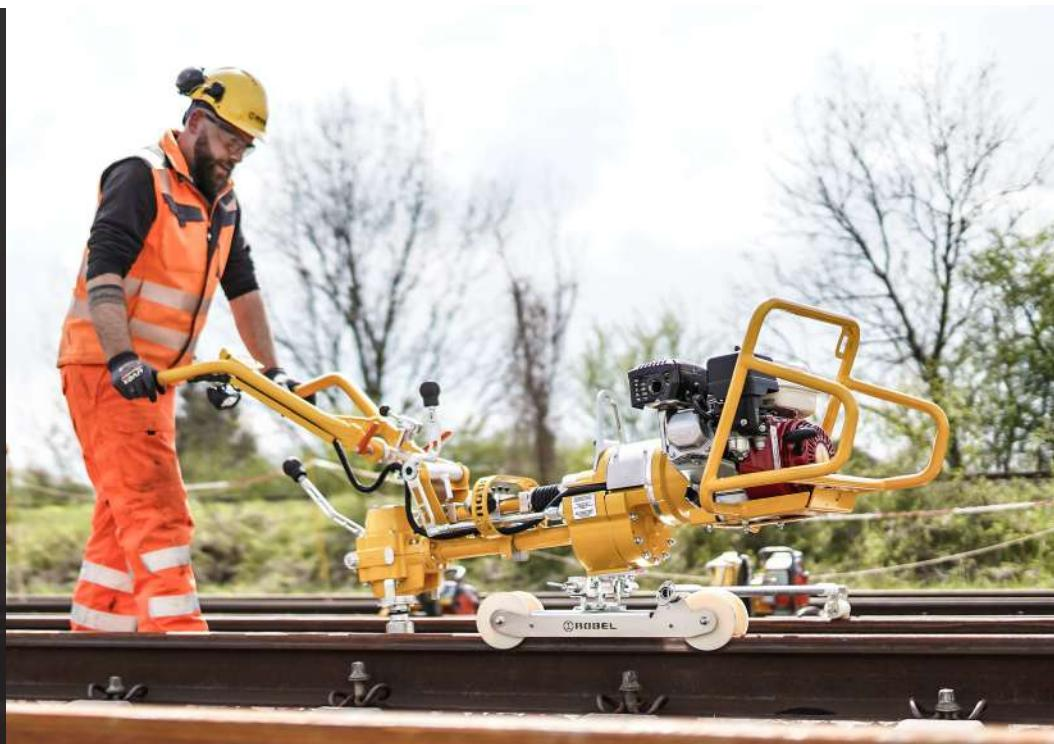
**For tightening and loosening lag screws.**
