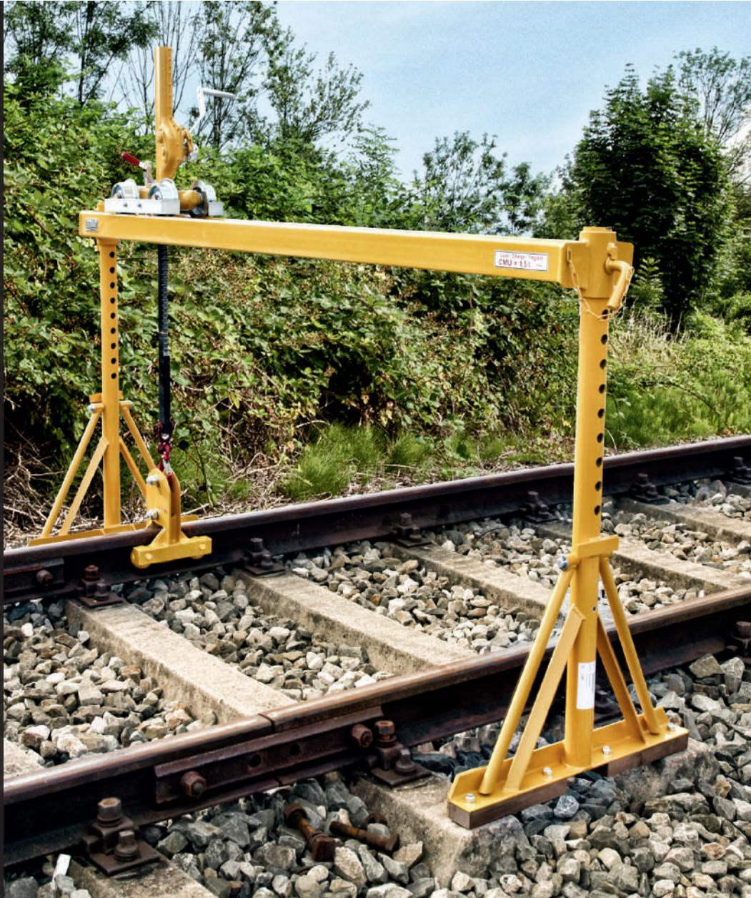
For lifting rails and moving rails longitudinally and laterally.
