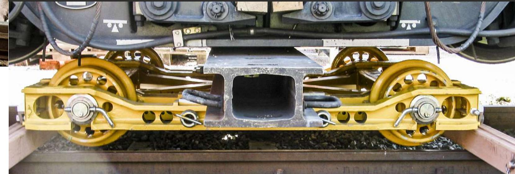
**For recovering and transporting rail vehicles with defective wheels or wheel sets.**
