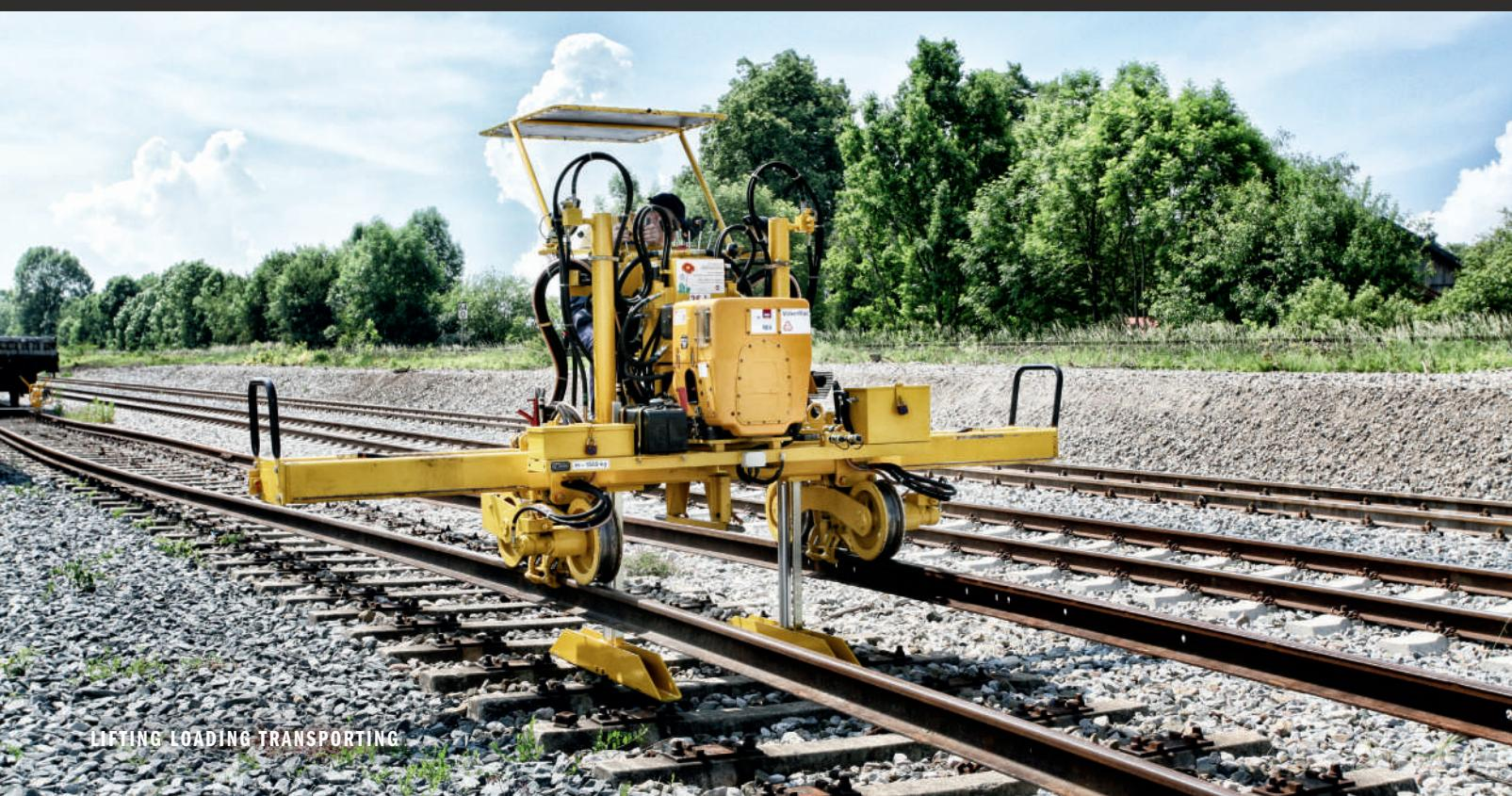
For continuous gradual repositioning of rails to the desired track gauge.
