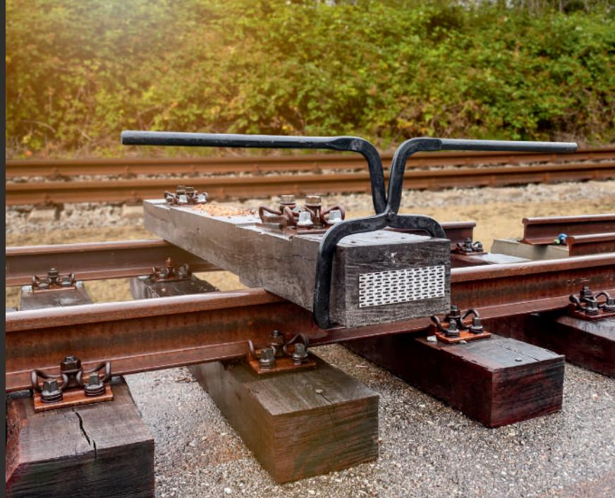
For lifting ties manually.
