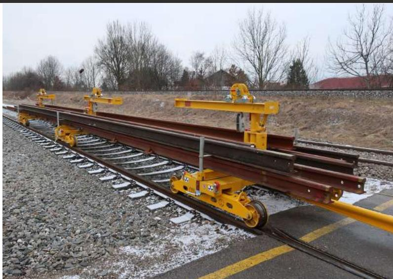
**Safe transport on four-wheeled chassis with rail loader and trolley.**
