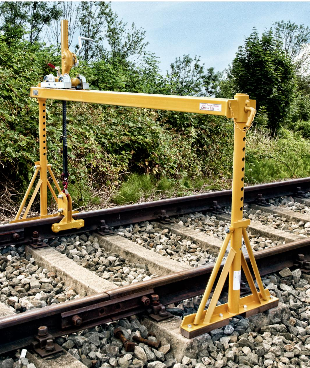
For lifting rails and moving rails longitudinally and laterally.
