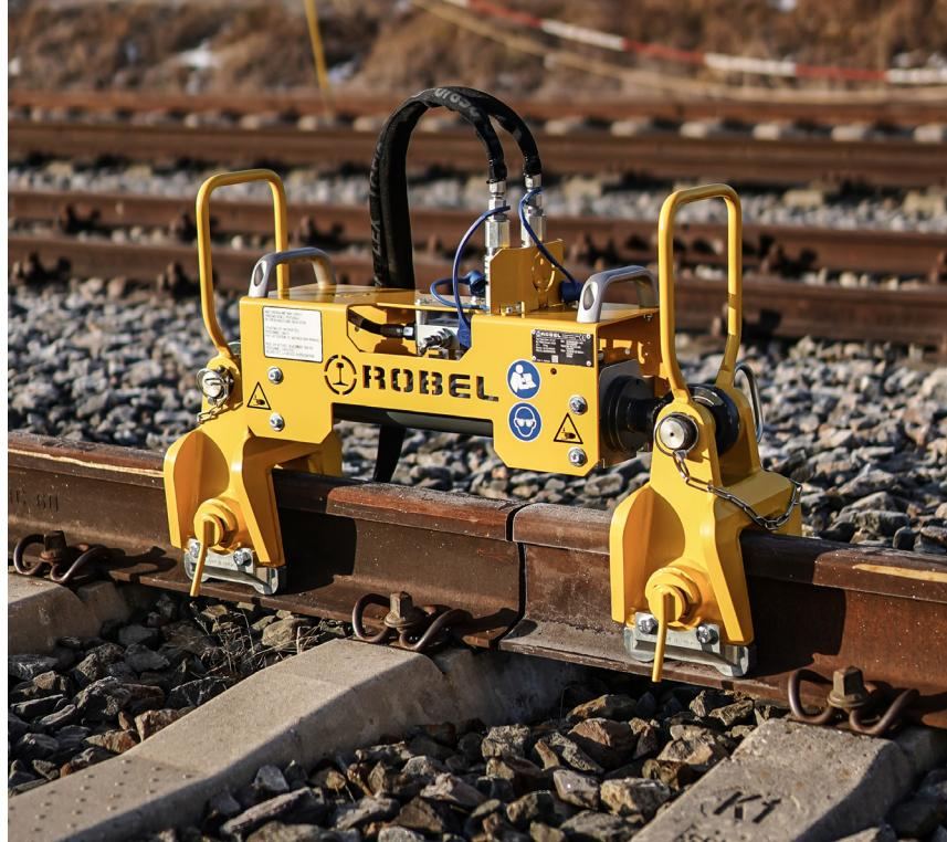
Designed for pulling and pushing running rails.
